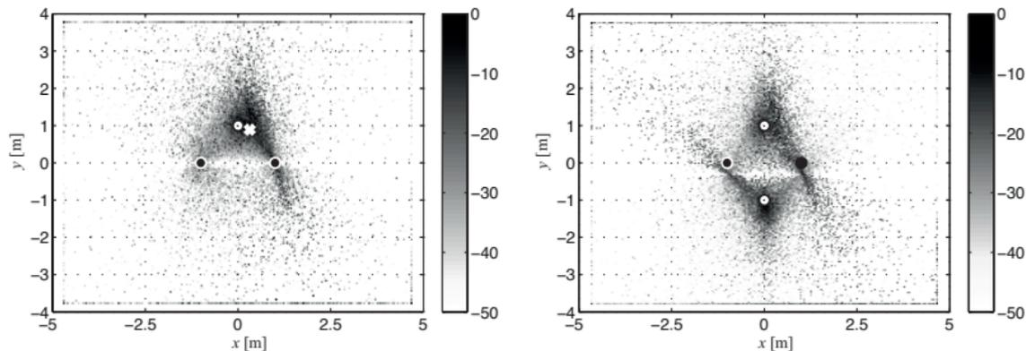
**Figure :** Spatial power density obtained using two circular arrays ( $M = 4$  and  $r = 1.6$  cm) for a one talker (left) and two talkers (right).
