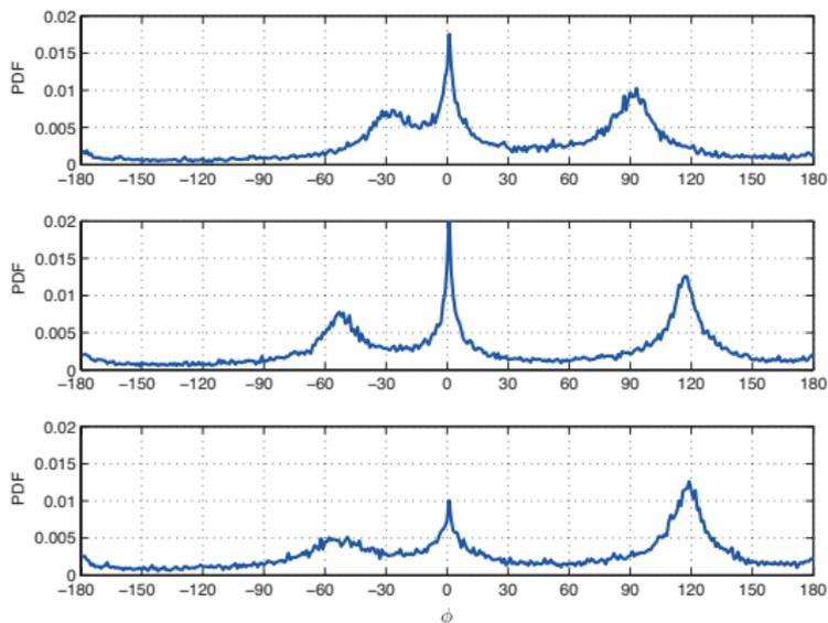
**Figure :** Probability density function (PDF) of the azimuth for the given scenario of three simultaneously active talkers [Schultz-Amling et al., 2010]. Top: Microphone at position  $p_1$ . Middle: Microphone at position  $p_2$ . Bottom: Microphone at position  $p_1$  and virtually moved to  $p_2$  with the acoustical zoom processing.
