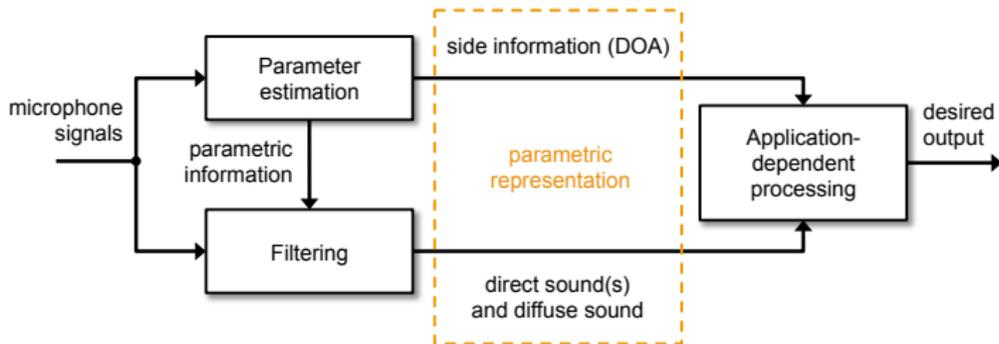
Figure : Parametric spatial audio processing scheme.
