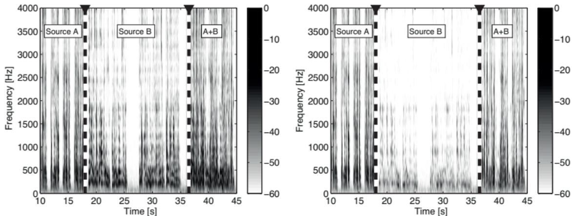
**Figure :** Spectrogram of a virtual omnidirectional microphone signal (left) and a virtual cardioid microphone pointing to Source A (right).
