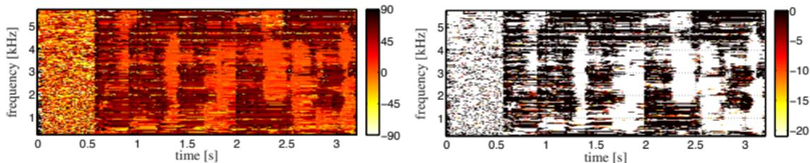
Figure : Left: DOA  $\varphi_1(k, n)$  as a function of time and frequency. Right: Desired response  $|G(k, \varphi_1)|^2$  in dB for DOA  $\varphi_1(k, n)$  as a function of time and frequency.
