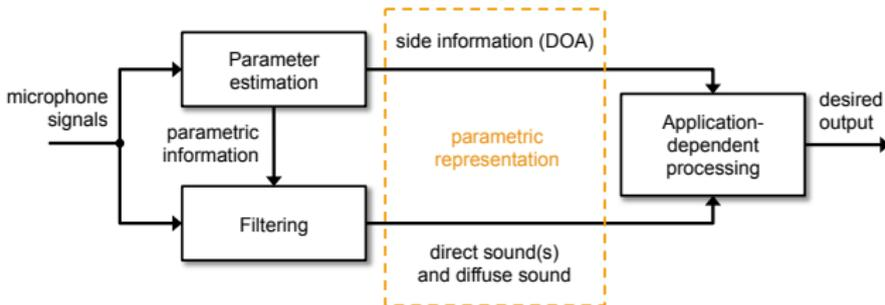
Figure : Parametric spatial audio processing scheme.
