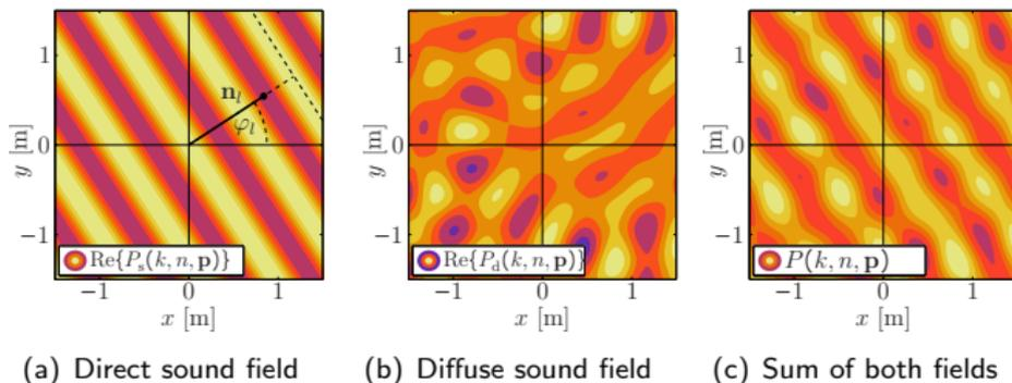
**Figure :** Example of a single plane wave, a diffuse field, and the sum of both fields.
