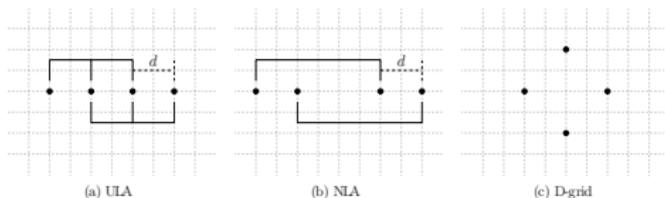
Figure : Typical microphone setups in practice.
