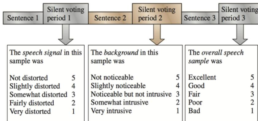
**Figure:** The ITU-T P-835's scheme for evaluating the subjective quality of speech enhancement algorithms. Each test sample is comprised of three subsamples, where each subsample is followed by a silent voting period.
