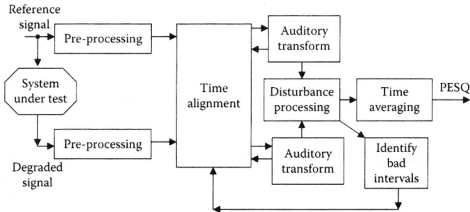
Figure: Block diagram PESQ measure [Loizou, 2007]
