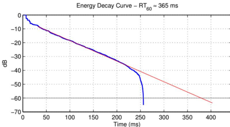
Figure: Determining the reverberation time.
