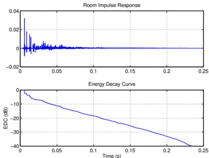
**Figure:** Example of an energy decay curve.
