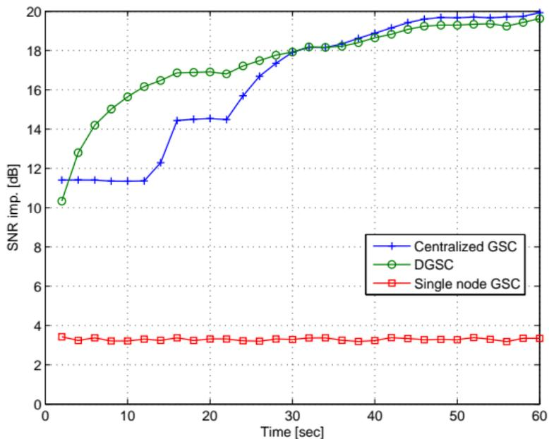
The convergence of the tested algorithms versus time.
