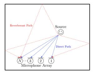
Figure 5: Illustration of the reverberant model of signal propagation.
