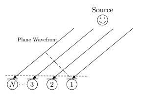
Figure 4: Illustration of the free-field model of signal propagation.
