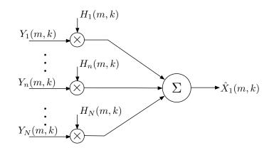
Figure 6: General block diagram for a beamformer.
