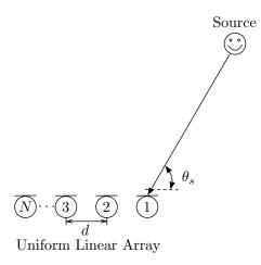
Figure 8: Reference diagram for Lab Experiment 1.  $\theta_s$  is the angle of incidence of the desired source, d is the inter-microphone distance and N is the total number of microphones of the ULA. In practice,  $\theta_s$  is computed with respect to the center of the array.
