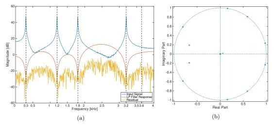
Figure 10: Linear prediction in the frequency- and z-domains. Depicted for a prediction order of 10. Figure (a) depicts the input signal, the filtered signal and the linear prediction filter response in the frequency domain. The dashed lines illustrate the exact positions of the roots of the filter. Figure (b) shows the roots of the linear prediction filter on the z-plane.
