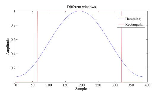
Figure 7: Illustration of the two windows.
