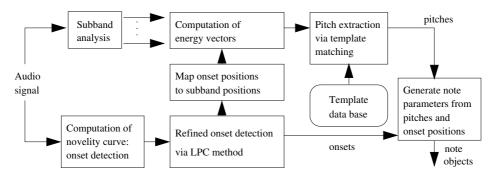
Figure 5: Diagram of the feature extraction algorithm.
