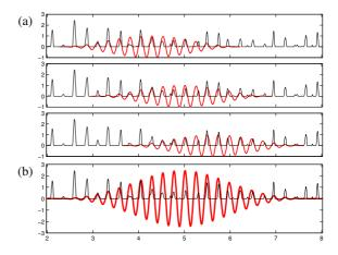
**Figure 2:** (a) Optimal sinusoidal kernel  $\kappa_t$  for various time parameters t using a kernel size of 4 seconds for the novelty curve shown in Fig. 1d. (b) Accumulation of all kernels. From this, the PLP curve  $\Gamma$  (see Fig. 1f) is obtained by half-wave rectification.
