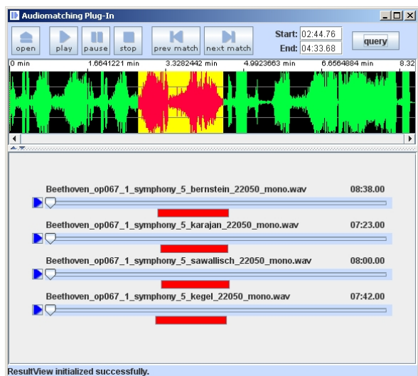
Fig. 1: Result of fragment-level content-based audio retrieval. Top: Query (yellow background) consisting of an audio fragment. Bottom: Retrieval result consisting of different performances.
