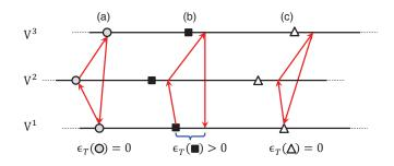
Fig. 1. Illustration of the concept of a triple error on the time axis of three different versions  $V_1$ ,  $V_2$ , and  $V_3$ . The red arrows indicate alignments between the different versions. The circles, squares and triangles mark corresponding ground-truth positions in the different versions. The triple error is denoted by  $\epsilon_T$ . (a) Consistent alignment with triple error of zero. (b) Inconsistent alignments with a triple error.
