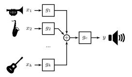
Figure 2: Audio Engine Overview.  $x_1, \ldots, x_k$  denote inputs,  $g_1, \ldots, g_k$  denote individual gain nodes,  $g_c$  denotes common gain node,  $g_c$  denotes output
