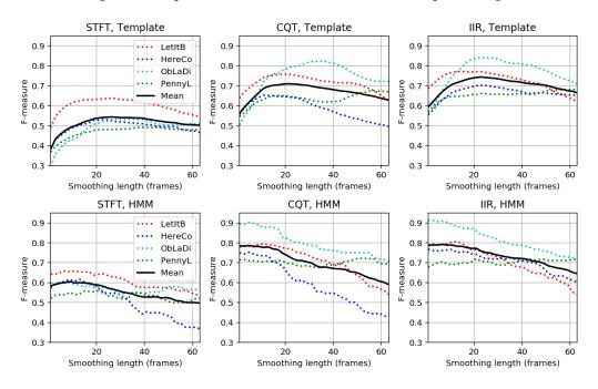
**Figure 14.** Prefiltering experiments for a template-based and an HMM-based chord recognizer applied to three different input chroma representations (STFT, CQT, IIR). The evaluation is performed on the basis of four Beatles songs (LetItB, HereCo, ObLaDi, PennyL).
