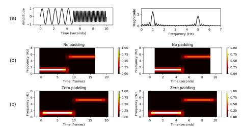
**Figure 8.** (a) Time-domain signal (using a sampling rate  $F_s = 256$ ) and magnitude Fourier transform. (b) STFT (N = 512, H = 128) without padding. (c) STFT (N = 512, H = 128) with zero-padding.
