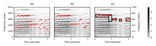
**Figure 23.** Salience representation with trajectories computed by (**a**) a frame-wise approach, (**b**) an approach using continuity constraints, and (**c**) a score-informed approach.
