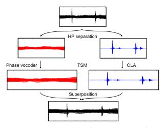
**Figure 21.** Application of HPS for time–scale modification (TSM), where TSM based on the phase vocoder is used for the harmonic component and TSM based on OLA (overlap-add techniques) is used for the percussive component (see [53]).
