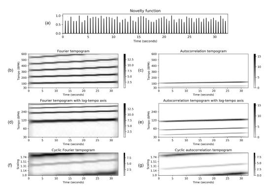
**Figure 16.** Different tempogram representations of a click track with increasing tempo (110 to 130 BPM). (a) Novelty function of click track. (**b**,**d**,**f**) Fourier tempogram with linear/logarithmic/cyclic tempo axis. (**c**,**e**,**g**) Autocorrelation tempogram with linear/logarithmic/cyclic tempo axis.
