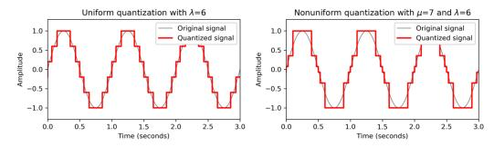
**Figure 9.** Uniform and nonuniform quantization (based on  $\mu$ -law encoding) using  $\lambda = 6$  quantization levels.
