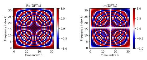
**Figure 7.** The matrix  $DFT_N$  and a visualization of its real and imaginary parts for the case N = 32.
