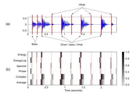
**Figure 15.** Excerpt of "Another One Bites the Dust" by Queen. (a) Waveform representation and annotated note onsets (from [1], Figure 6.1a) (b) Comparison of novelty detectors using a matrix-based visualization.
