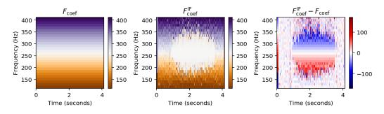
**Figure 22.** Interpretation of time–frequency bins of an STFT as specified by the (frame-independent) frequency values  $F_{\text{coef}}(k)$  and the (frame-dependent) instantaneous frequency values  $F_{\text{coef}}^{\text{IF}}(k, n)$ . The bin offset (specified in Hertz) is given by  $F_{\text{coef}}^{\text{IF}} - F_{\text{coef}}$ .
