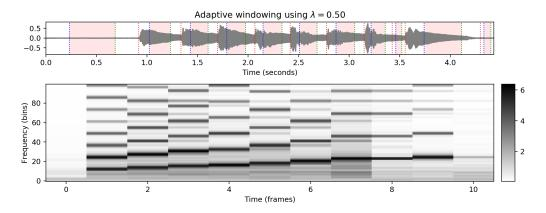
**Figure 17.** Example of adaptive windowing using a parameter  $\lambda \in \mathbb{R}$  to control the neighborhood's relative size to be excluded. (**Top**): Waveform and nonuniform time grid (indicated by red vertical lines). (**Bottom**): Adaptive feature representation (obtained from a spectrogram) with frames corresponding to the shaded segments of the signal.
