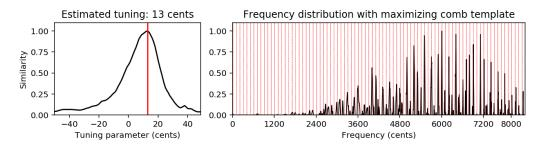
**Figure 10.** Tuning procedure using a comb-filter approach. **Left**: Similarity function with maximizing tuning parameter at 13 cents. **Right**: Frequency distribution (with logarithmic frequency axis) and maximizing comb template (shown as red vertical lines).
