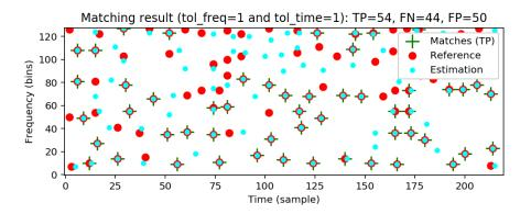
**Figure 18.** Evaluation measures that indicate the agreement between two constellation maps computed for an original version (Reference) and a noisy version (Estimation).
