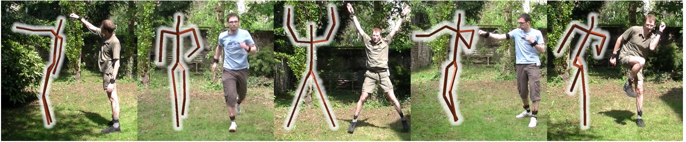
Fig. 5: Using accelerations obtained by four 3D accelerometers attached to a human actor as control input, a full-body animation is reconstructed using motion fragments retrieved from a knowledge base consisting of motion capture data.
