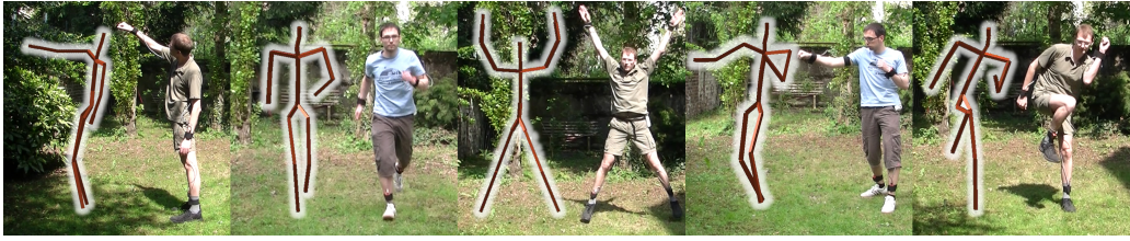
Figure 3.13: Frames taken from the video illustrating our outdoor motion reconstruction experiment. The motion synthesis was driven by four 3D accelerometers attached to the lower arms and lower legs of one of two actors. Reconstructed poses are always shown to the left of the original performance.
