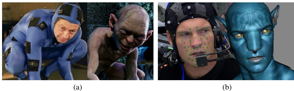
Figure 1.2: Marker based Motion Capture: a series of markers are tracked by several cameras to reconstruct the 3D motion. We show making-off of the movies (a) The Lord of the Rings , and (b) Avatar . 2
