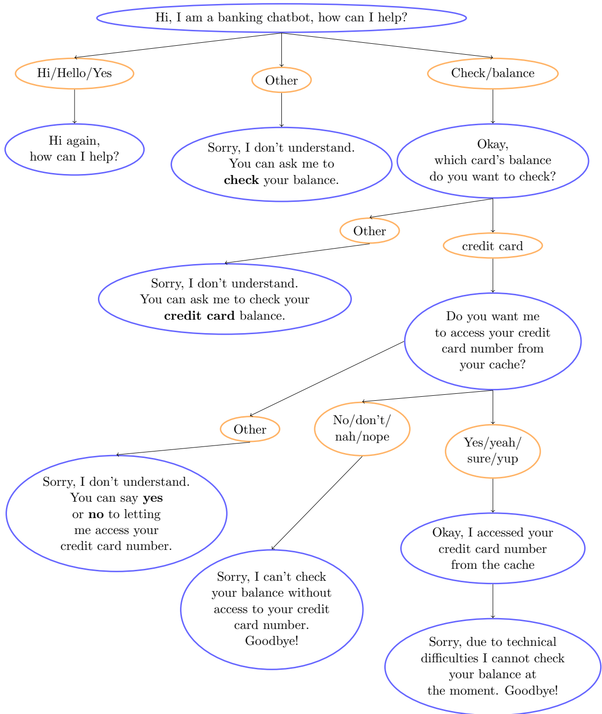
Figure A.2: Dialogue Tree for the banking scenario in the access condition, blue circle show the chatbot, orange circles show the possible inputs for the user.
