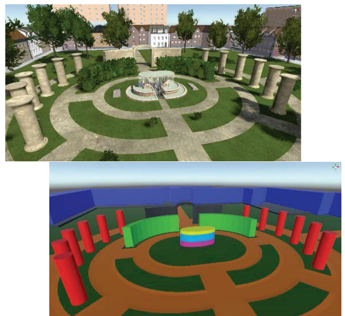
Figure 3: Visual and acoustic materials. Each mesh face can be defined with acoustic properties. This allows the calculation of reflections, coupling between rooms, acoustic transmission through e.g., closed doors and occlusion.
