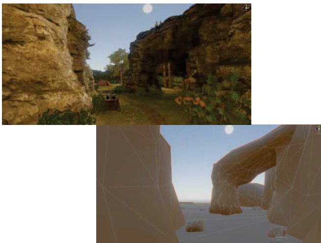
Figure 2: Visual and acoustic geometry. For the acoustical rendering not all details of the visual rendering are necessary.
