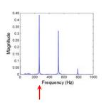
Analysis using sinusoid with 262 Hz
